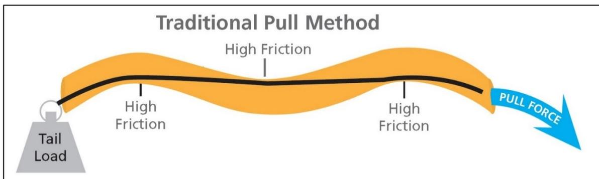
**Figure 5: Traditional Pulling Method (not to scale)**
